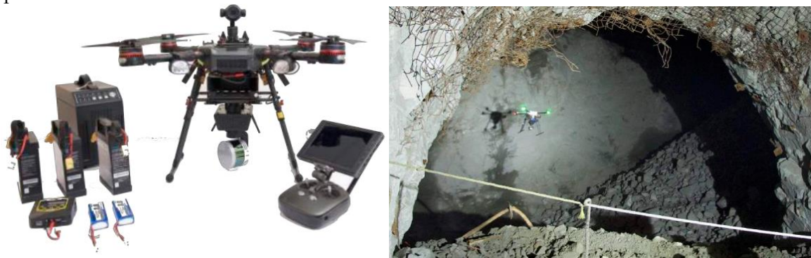
Figure 1. A) - The Hovermap used throughout the trials. B) Flying through an open draw point into a large stope
