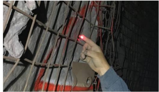
Figure 3. (a) A survey sphere is placed on the wall. (b) Either the collar or the sphere centroid location is known so the point cloud can be referenced to these locations
