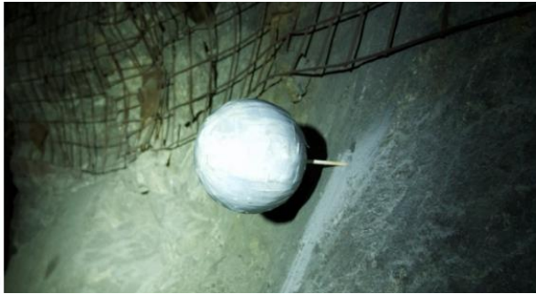
Figure 3. (a) A survey sphere is placed on the wall. (b) Either the collar or the sphere centroid location is known so the point cloud can be referenced to these locations
